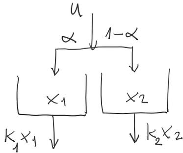
$$\begin{aligned} \dot{x}_1 &= \alpha u - K_1 x_1 \\ \dot{x}_2 &= (1-\alpha) u - K_2 x_2 \end{aligned} \quad A = \begin{bmatrix} -K_1 & 0 \\ 0 & -K_2 \end{bmatrix}, \quad b = \begin{bmatrix} \alpha \\ 1-\alpha \end{bmatrix}$$
