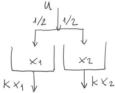
$$A = \begin{bmatrix} -K & 0 \\ 0 & -K \end{bmatrix}, \quad b = \begin{bmatrix} 1/2 \\ 1/2 \end{bmatrix}, \quad R = \begin{bmatrix} 1/2 & -K/2 \\ 1/2 & -K/2 \end{bmatrix}, \quad X_r = \left\{ \begin{bmatrix} 1/2 \\ 1/2 \end{bmatrix} \right\}$$
