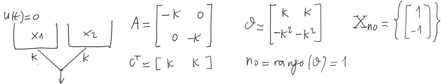
Scelgo  $T$  e ricavo  $T^{-1}$ , con  $z_1 = z_0 = \underbrace{[1 \quad 1]}_{\perp X_{no}} x = x_1 + x_2$  e  $z_2 = z_{no} = \underbrace{[1 \quad 0]}_{\text{non } \perp \text{ a } X_{no}} x = x_1$
