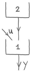
$$\begin{aligned}\dot{x}_1 &= u + k_2 x_2 - k_1 x_1 \\ \dot{x}_2 &= -k_2 x_2 \\ y &= k_1 x_1\end{aligned}$$
